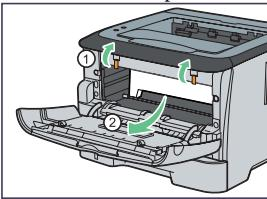
BXG014 | 5. Remove the protective material attached inside the printer.<br>
